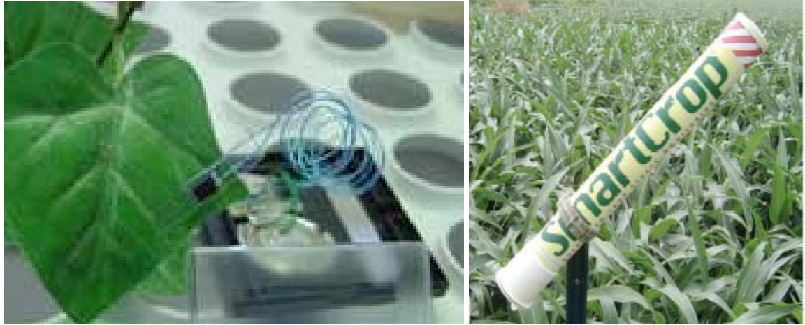
Figure 5: AgriHouse leaf thickness sensors (left) and Accent Engineering SmartCrop leaf surface temperature sensors (right): systems of these in-field sensors monitor real-time plant conditions and communicate this data wirelessly to a central server... or a cell-phone! (Leaf sensor photo from Colorado company AgriHouse Inc., based on technology developed at University of Colorado at Boulder; SmartCrop photo from Texas company Accent Engineering, Inc., based on technology developed by the U.S.D.A. Agricultural Research Service)
